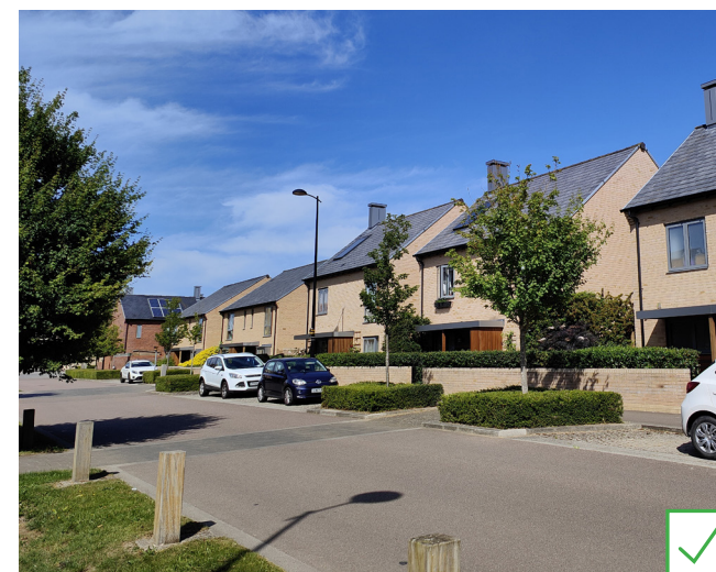
Street bollards and hedge planting prevent inappropriate parking
