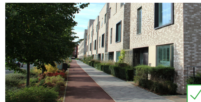
Rain gardens can help intercept and filter surface run-off
